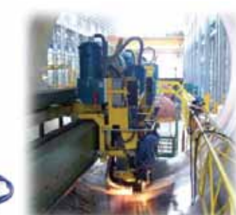
ESW Cladding System
